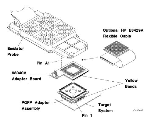
4 Connect the auxiliary power cable from the front of the HP 64700A/B Mainframe to the 68040V adapter board.
