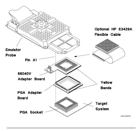
**3** Align pin A1 of your emulator probe with pin A1 on the 68040V adapter board. Attach the emulator probe as shown.
