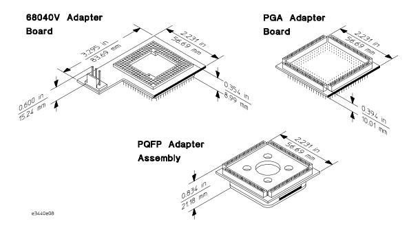
The HP E3440A 68040V Adapter allows the HP 64783A 68040 Emulator, to be used with a 68040V target system. It adapts the 68040V pin-out to that of the 68040 processor and also provides signal and power supply translation from 3.3V to 5V.
